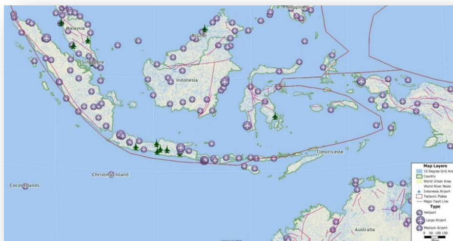
FIGURE 5. GIS platform allows to overlap information on key operational infrastructure (e.g. airports –civil and military), tectonic plates and fault lines
