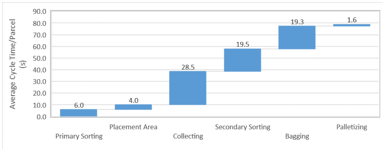
Figure 5.1. Example of Using Time Motion Studies and Value Stream Mapping to Determine Warehouse Operation Bottlenecks
